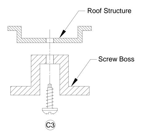
Note: If longer screws are substituted, care should be taken to prevent piercing the roof, and be sure that pan head screws and washers are used to prevent screws from pulling through the screw boss. Eight screws <u>must</u> be used and secured to solid structure when mounting.
